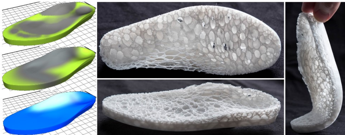
Figure 1: Illustration of a shoe insole with varying elasticity, modeled using a porous pattern that can be manufactured on filament printers [5].
